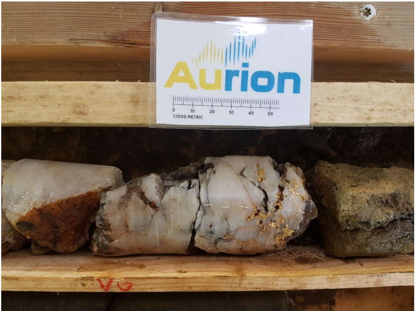
Coarse visible gold in drillhole AM18042
