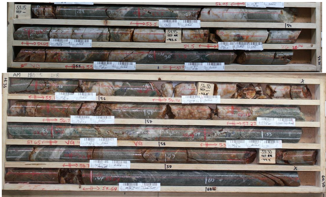
Aamurusko Main; Drillhole AM18035. 12.45 g/t Au over 5.2 m from 53.5 to 58.7 m
