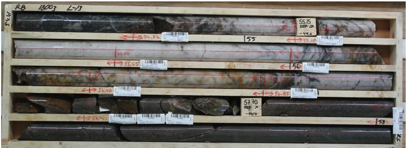
Aamurusko West; Quartz vein in drillhole RB18003; assays pending
