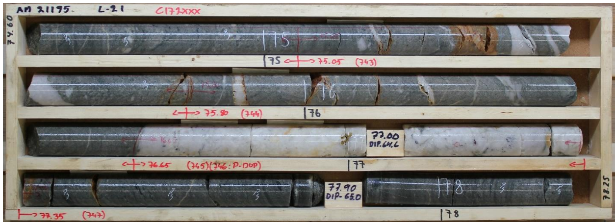
Photo 1. AM21195, NW Zone. High grade vein (70.1 g/t Au over 0.70 m) within lower grade (0.1-0.2 g/t Au) interval hosted by sericite and silica altered clastic sediment with pyrite dissemination.
