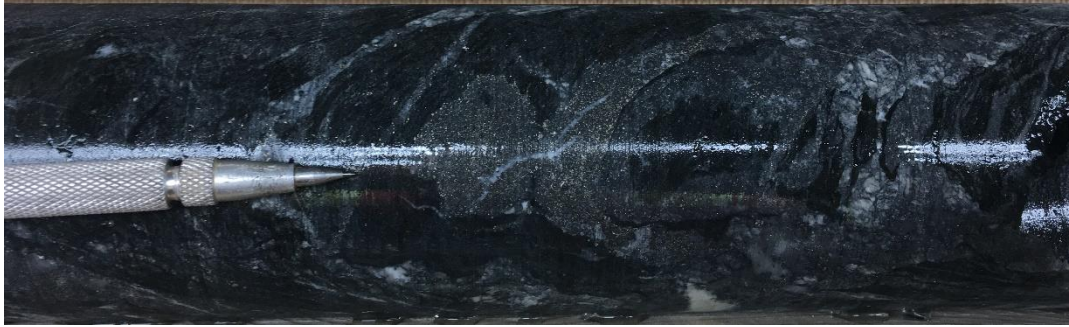
IKK21006, 125.0 m. Gold grade 6.75 g/t. Magnetite-chlorite-biotite altered ultramafic rock with pyrite and magnetite veinlets.
