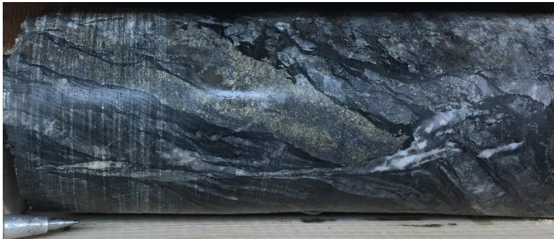
IKK21006, 127.0 m. Gold grade 1.70 g/t. Magnetite-chlorite-biotite altered ultramafic rock with pyrite and magnetite veinlets.
