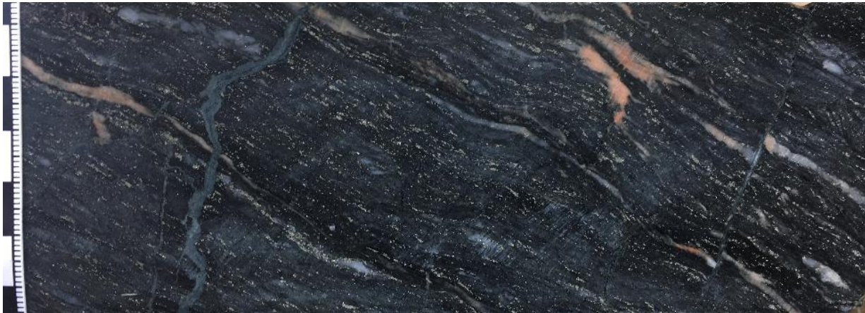
Figure 7: IKK21010, 184.0 m. Gold grade 1.55 g/t. Interfolial pyrite in chlorite-biotite-Kfeldspar altered felsic tuff.
