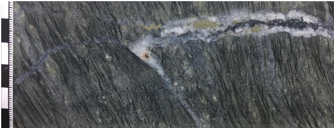
Figure 8: IKK21011, 97.7 m. Gold grade 1.18 g/t. FeMg-carbonate-chlorite-altered mafic volcanic with quartz-dolomite-magnetite-specular hematite-pyrite vein in mafic volcanic .
