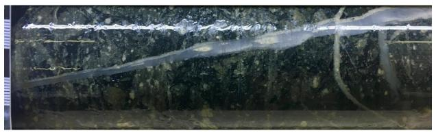
Figure 4: Drill hole KUE22027. Brecciated Fe-dolomite and Qtz veins in high strain silica-tourmaline breccia cut by Qtz and Fe-dolomite veinlets at 173.35 m within interval of 1.56 g/t Au over 24.8 m from 159.0 m.
