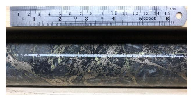
Figure 6: Drill hole KUE22028. Brecciated graphitic mudstone with abundant pyrrhotite, pyrite and chalcopyrite veinlets at 174.2m within interval of 0.26 g/t and 1.07 % Cu over 12.80 m.
