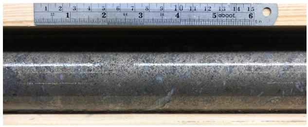
Figure 7: Drill hole KUE22028. Massive pyrrhotite vein at 225.1m within 6.25 g/t Au over 6.00 m
